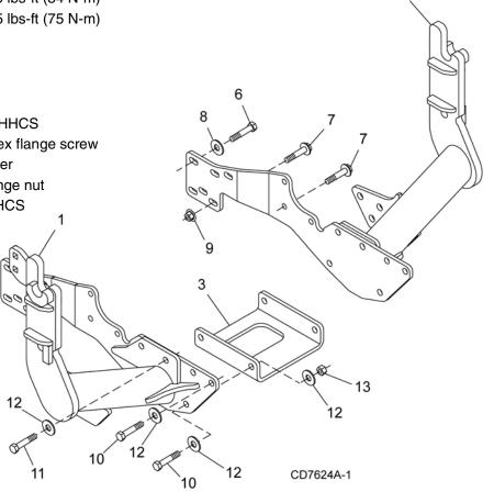
Figure 3. 2104045 Mount Kit Installation
